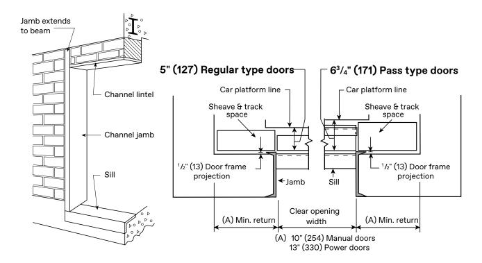
Note: All dimensions in parentheses are in millimeters unless otherwise indicated. Dimensional data shown here complies with the current ASME A17.1 and CSA B44 Safety Code for Elevators. Local codes may vary from the national codes. Consult your local TK Elevator representative for details.
