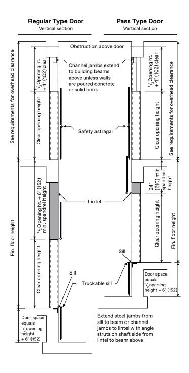
Note: All dimensions in parentheses are in millimeters unless otherwise indicated. Dimensional data shown here complies with the current ASME A17.1 and CSA B44 Safety Code for Elevators. Local codes may vary from the national codes. Consult your local TK Elevator representative for details.
