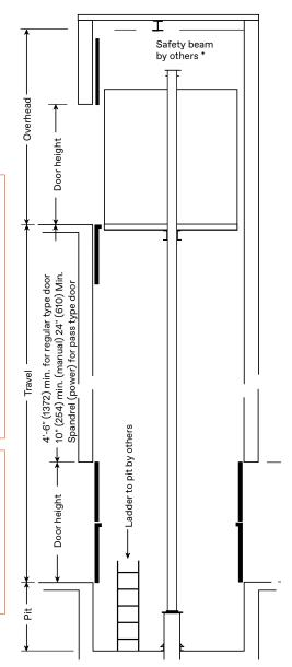
Safety beam required per OSHA 1926.502, provided and installed by others, as directed by TK Elevator local office. Clear overhead is shown to the bottom of the safety beam.
